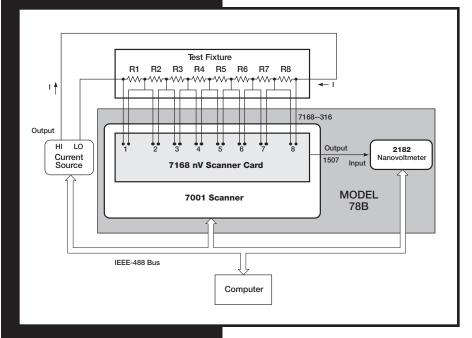
The Model 78B provides all instrumentation and accessories necessary to scan eight channels of the Model 7168 Nanovolt Scanner Card and make low-level voltage measurements.
